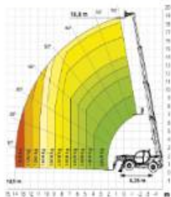
Load chart on stabilizers
