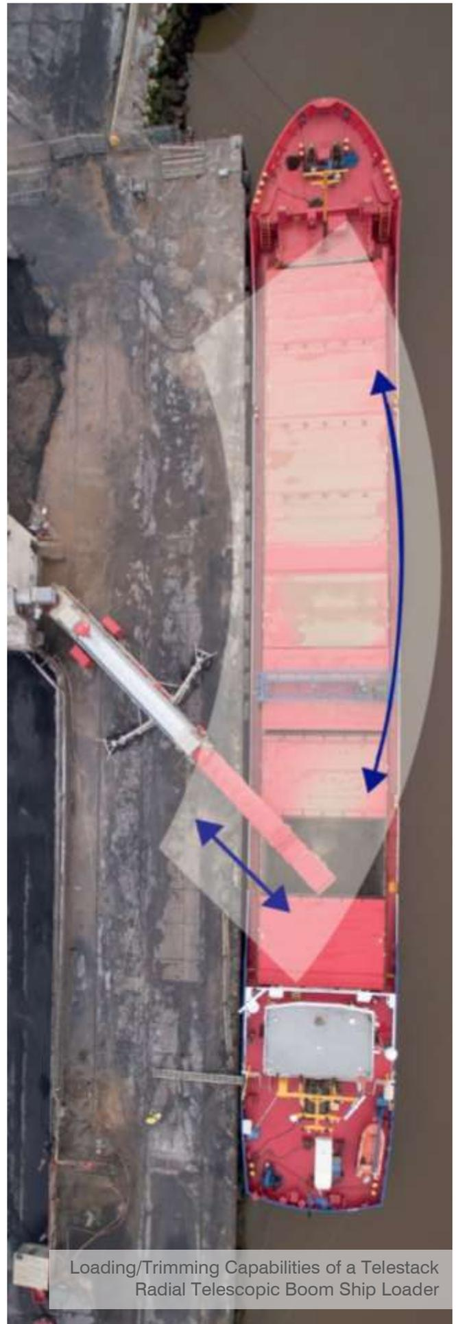
Loading/Trimming Capabilities of a Telestack Radial Telescopic Boom Ship Loader
